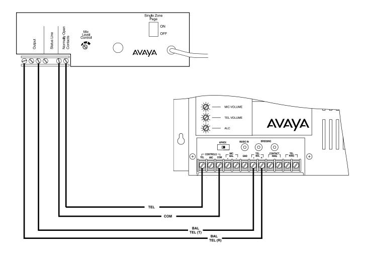
Figure 4. Typical Connections to a Telephone Paging Amplifier
